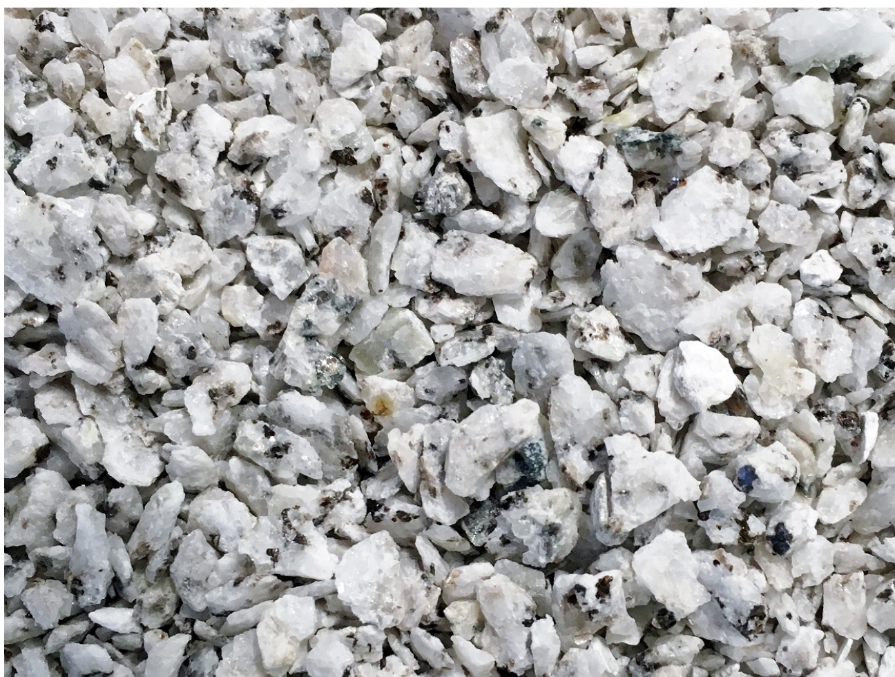
Granite drill cuttings from United Downs borehole (taken at 2140m depth) – chips approx. 2-3mm in size. Photo courtesy of Dr Robin Shail, Camborne School of Mines
