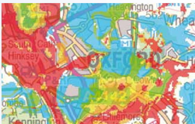
BGS Groundwater flooding susceptibility map
