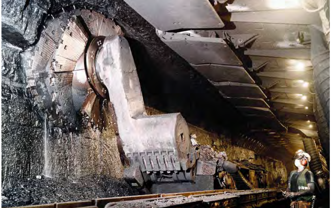
A coal cutting machine shearing a two metre thick slice from the Warwickshire Thick seam at Daw Mill Colliery in the West Midlands. Picture courtesy of MRP Photography.
