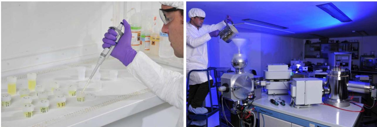
**Left: Uranium is purified from dissolved minerals. Right:  $^{238}\text{U}/^{235}\text{U}$  is measured with a mass spectrometer.**
