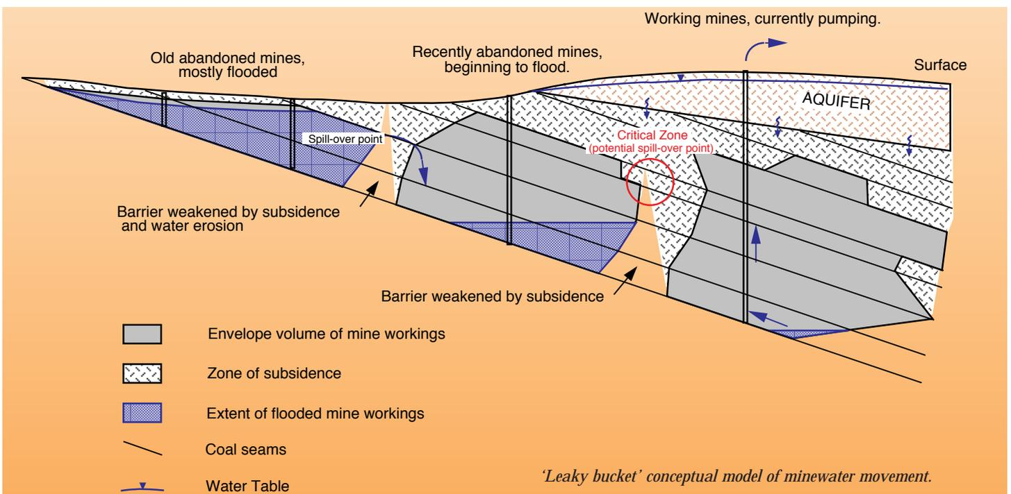
*‘Leaky bucket’ conceptual model of minewater movement.*
