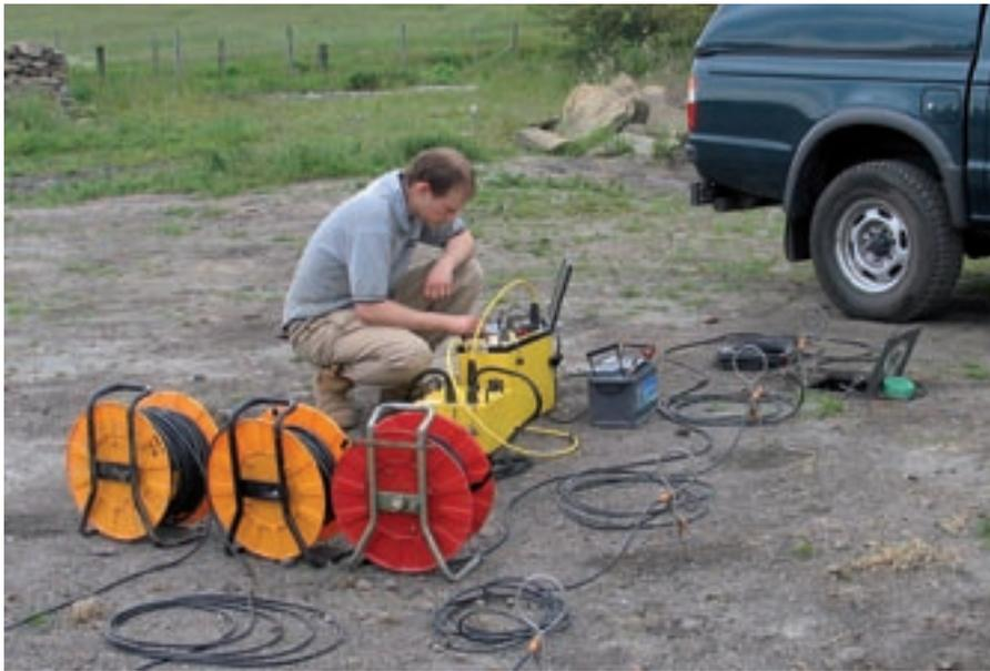
*A resistivity imaging survey in progress.*
