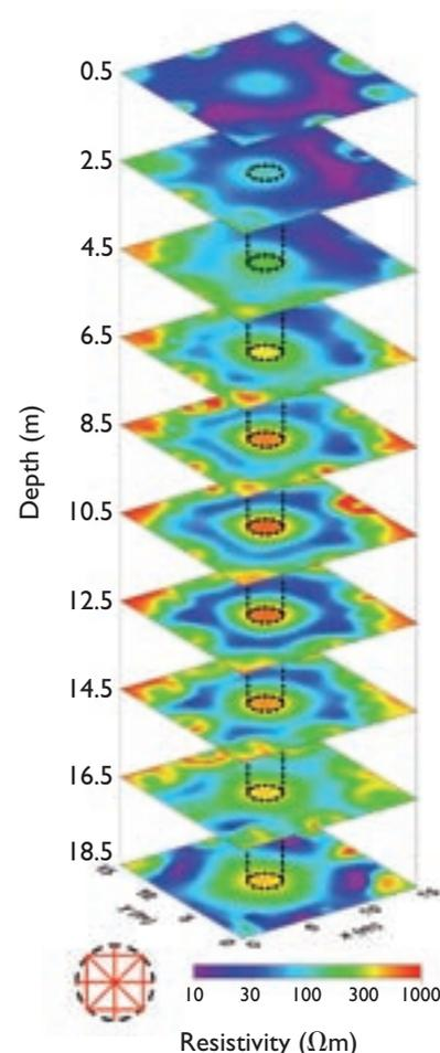
*A 3D resistivity image of a mineshaft. The central resistive feature in the image corresponds closely to the actual location and geometry of the air-filled shaft (shown by the dashed lines).*
