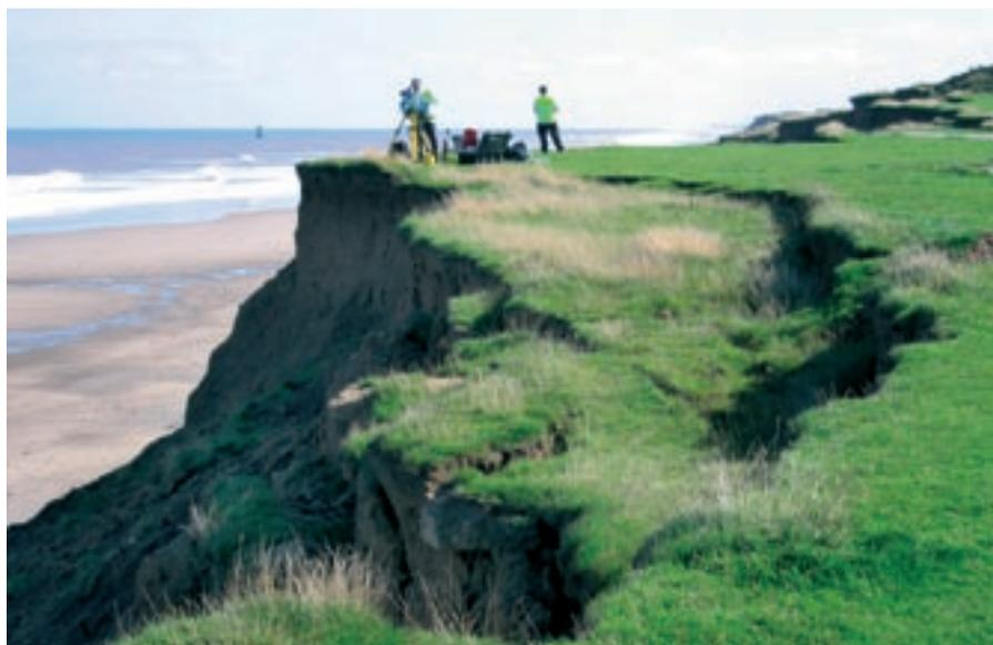
*Using a high-resolution laser scanner to measure landslide activity — the scanner helps to measure very small changes in the cliff surface which is vital in order to understand how the coast reacts to different climate patterns.*
