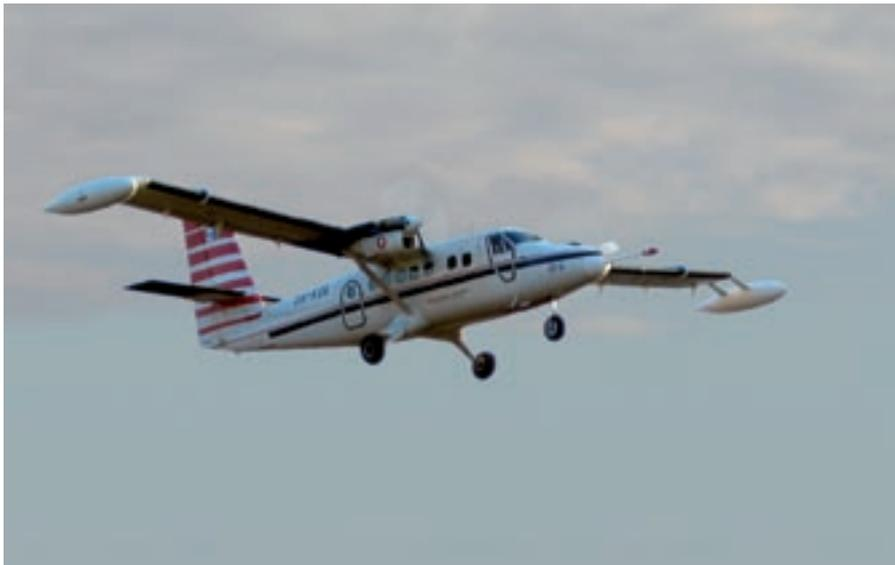
*The NERC Twin Otter aircraft, equipped with upgraded electromagnetic survey equipment, in operation during the TELLUS airborne geophysical survey project in Northern Ireland.*
