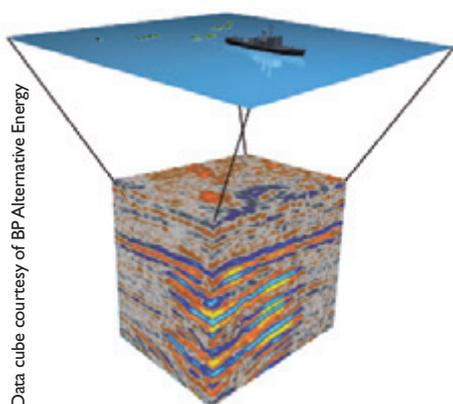
*Schematic view of a seismic survey operation with a 3D seismic 'cube' showing bright reflections corresponding to the CO<sub>2</sub> plume.*
