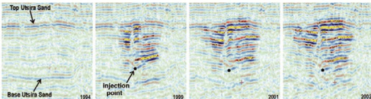
*Time-lapse seismic images from Sleipner showing vertical slices through the storage reservoir in 1994 prior to injection and through the expanding plume in 1999, 2001 and 2002. The total height of the plume is about 250 metres, with a total width in 2002 of around 2 km. (Images courtesy of BGS involvement in the SACS, SACS2 and CO2STORE projects).*
