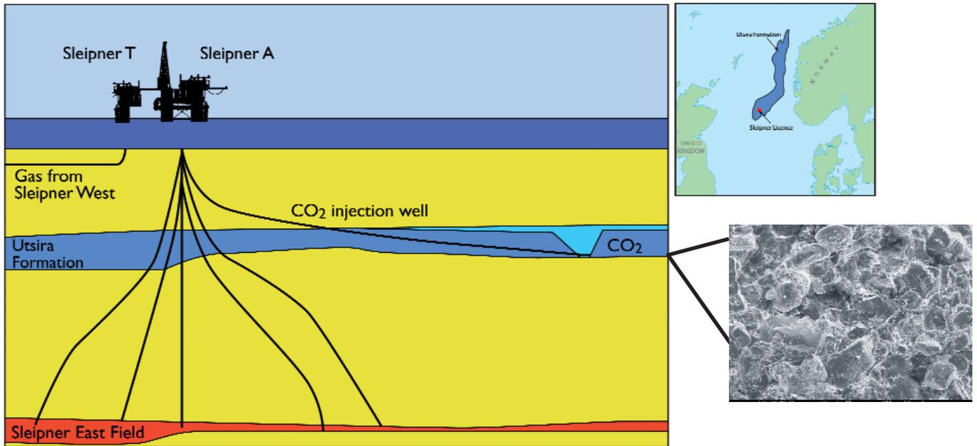
*Sleipner summary showing location map, cartoon of injection operation, and scanning electron microscope image of the porous Utsira Sand reservoir rock (images courtesy of Statoil and BGS).*
