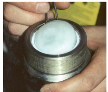
*Cylindrical sample of laboratory-grown CO<sub>2</sub> hydrate being removed from a steel pressure vessel.*
