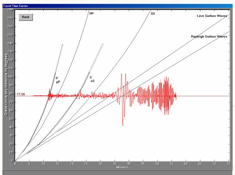
Amaseis has a useful feature that allows you to overlay a set of traveltime curves on your seismogram that can either be useful for
