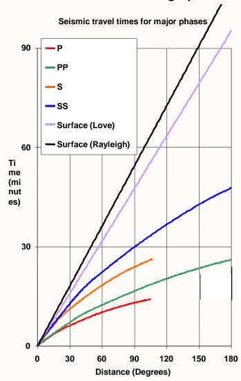
For a standard reference model of the Earth's velocity structure it is possible to calculate the theoretical arrival time of any particular ray-path (or seismic phase) for any given earthquake. A commonly used velocity model is called IASP91, a radially symmetrical velocity model where velocity varies only with depth. On the left is a
