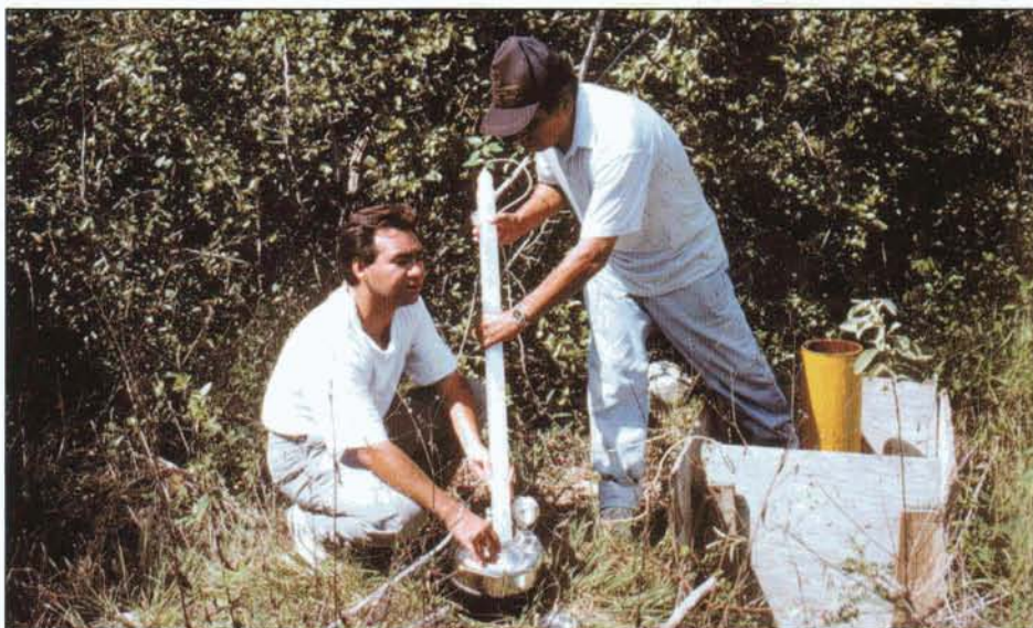
Sampling groundwater at a purpose built monitoring well.
