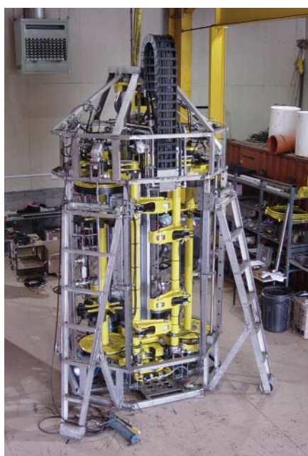
New BGS fifteen-metre sea-bed drill.
