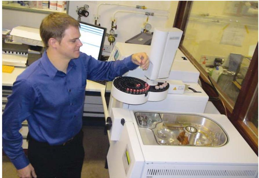
*Analysing estuarine sediments for endocrine disruptors using gas chromatography-mass-spectrometry-mass spectrometry (GC/MS/MS).*
