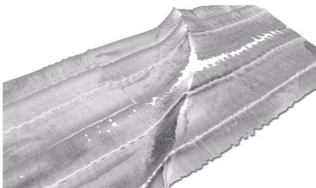
Sand wave: sidescan mosaic draped on multibeam surface.
