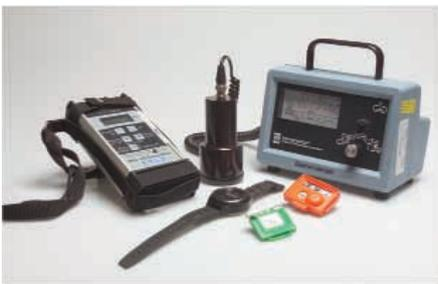
*Equipment used by staff working with radioactive materials for scanning new samples and for monitoring personal radiation doses.*
