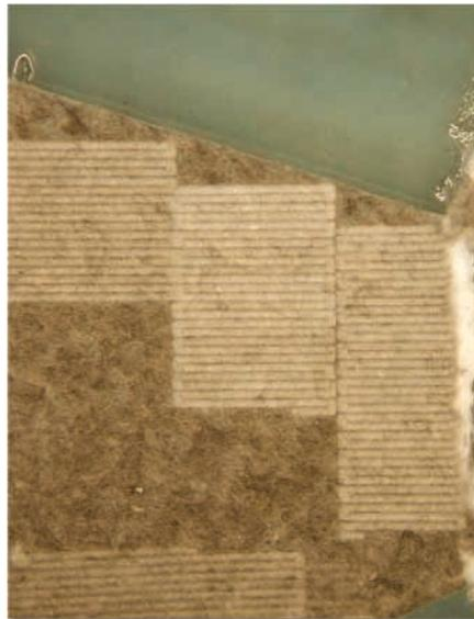
Photomicrograph of quartz-fibre filter, showing the raster sampling pattern produced by laser ablation during ‘dusting’ to remove the sample from the filter substrate. Width of each rastered line is 200 micrometres.
