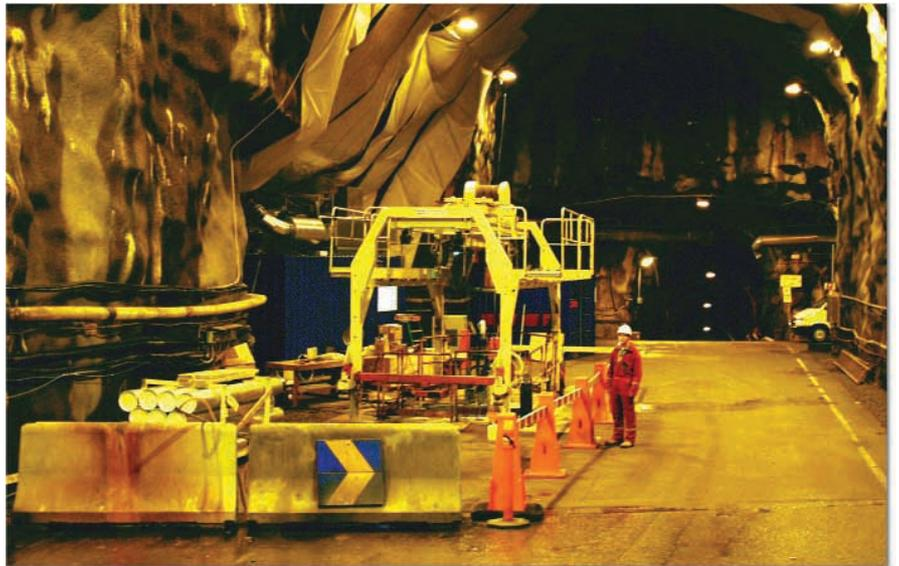
*Large scale gas injection test (Lasgit) 420m below ground at the Äspö Hard Rock Laboratory in Sweden. A BGS scientist stands next to a gantry crane positioned over the disposition hole.*
