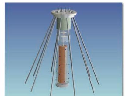
*Layout of the Lasgit experiment showing the copper canister, the bentonite buffer, the plug and the rock anchors.*
