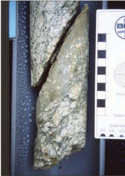
*A section of faultrock in the Cretaceous Toki Granite in borehole MIU-2 from the Mizunami Underground Laboratory site near Toki City, in Honshu, Japan.*
