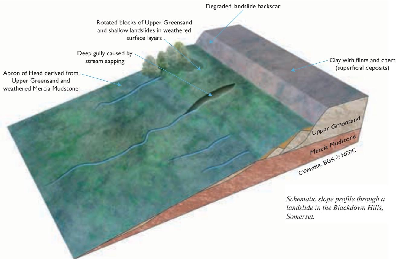
*Schematic slope profile through a landslide in the Blackdown Hills, Somerset.*
