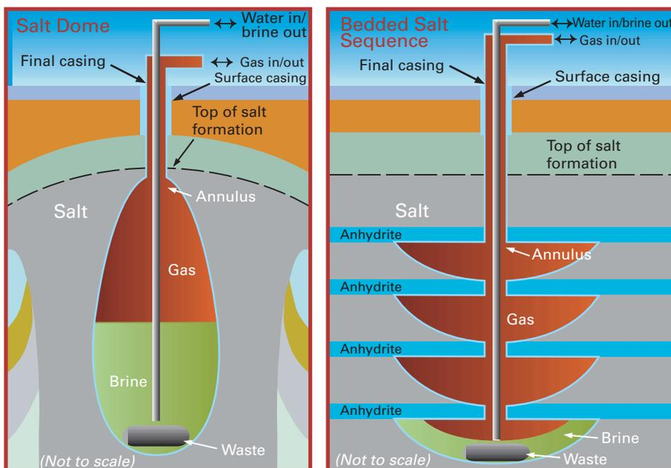
*Schematic of underground gas storage in salt caverns constructed in both salt domes and bedded salt sequences (normally the brine is displaced by gas before the cavern is brought into operation).*
