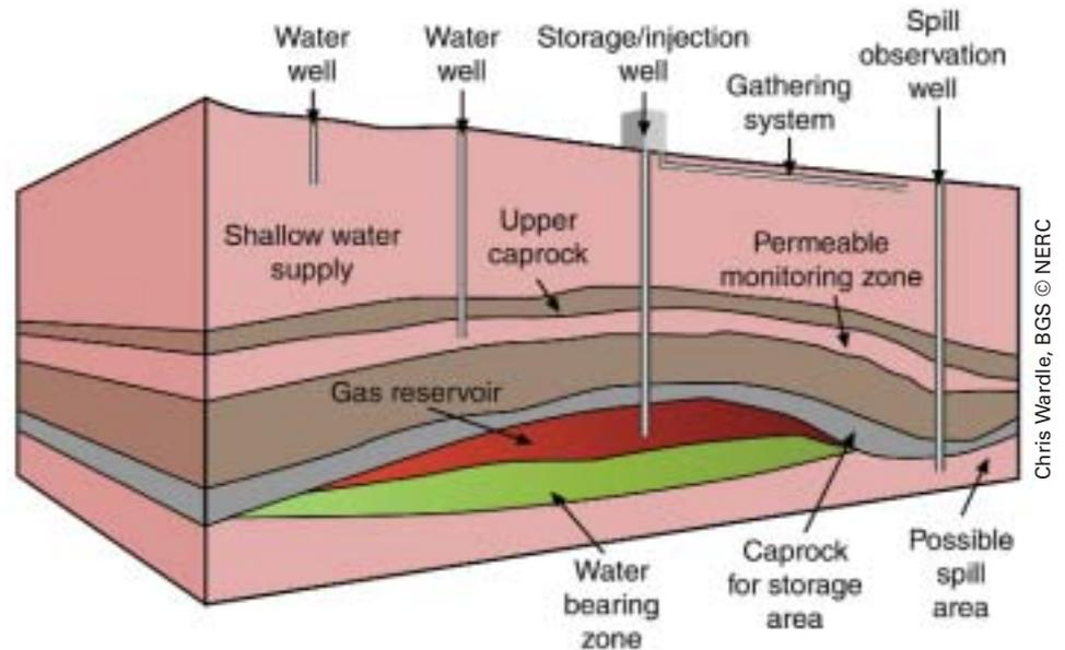
*Schematic representation of subsurface gas storage in depleted oil and gas reservoir.*
