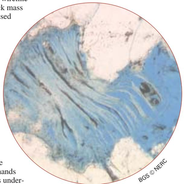
*Diagenetic alteration of mica grains in a sandstone reservoir causes increased porosity (stained blue). Field of view is five millimetres.*
