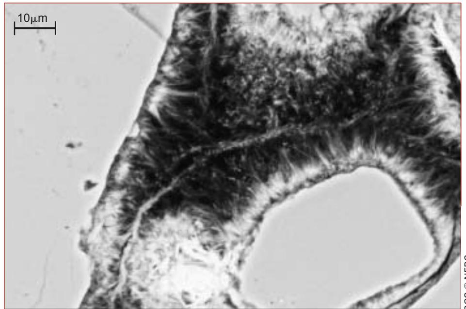
*Authigenic, fibrous illite cement destroys intergranular porosity in a sandstone reservoir (scanning electron microscope image).*
