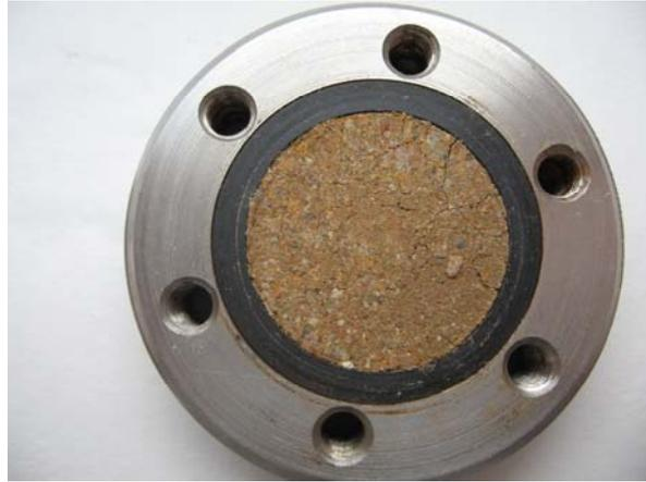
**Figure 9: Sample of saturated bentonite Rokle for measuring hydrogen migration**
