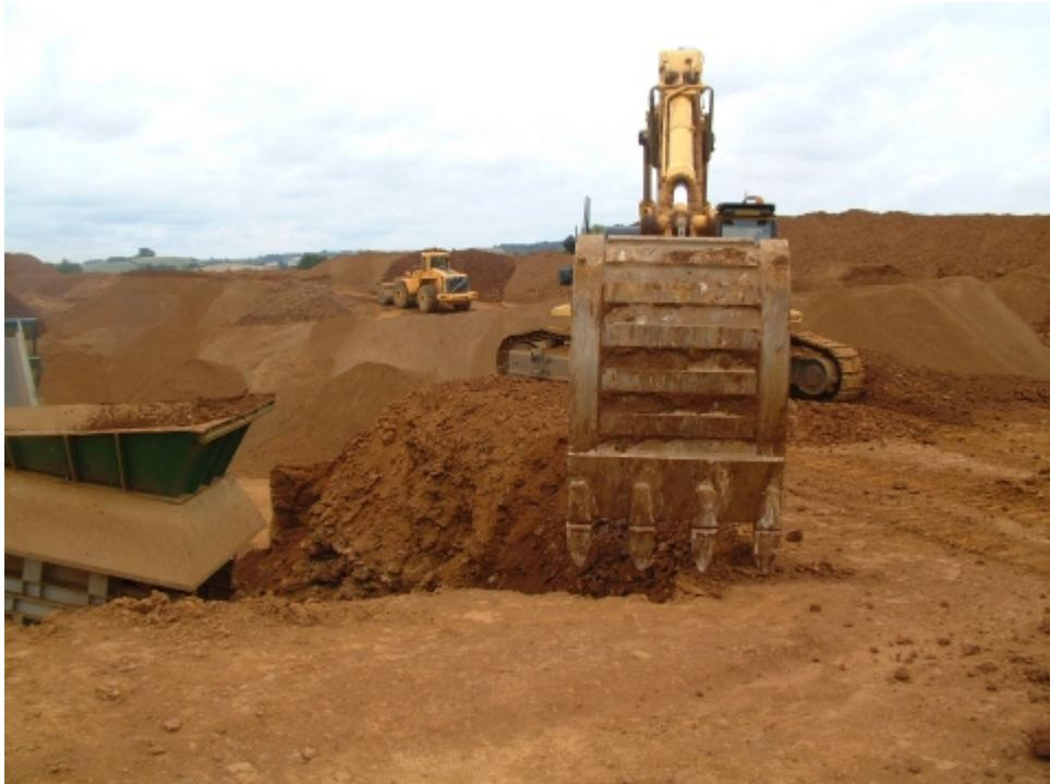
**Figure 2.** Marlstone Rock Formation ironstone being worked for crushed rock aggregate at Wroxton Fields Quarry near Banbury, Peter Bennie Ltd.
