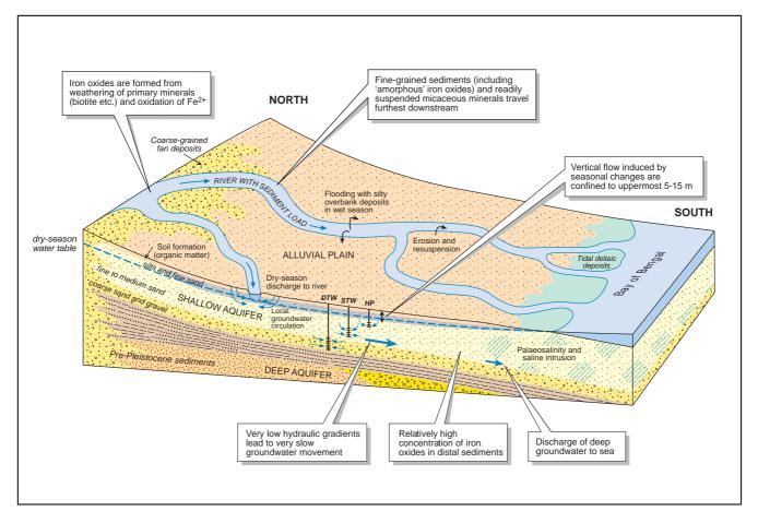
Figure 12.1. Block diagram showing the basic geology and hydrogeology of the Bengal Basin.
