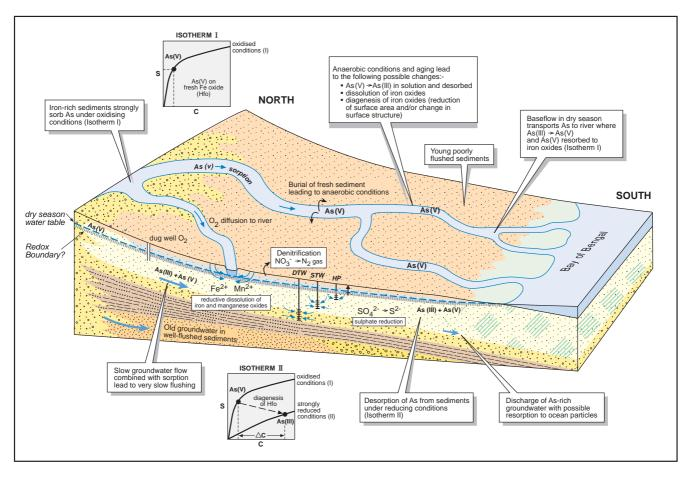
Figure 12.2. Block diagram showing the principal geochemical processes involved in the development of arsenic-contaminated groundwater in the Bengal Basin.
