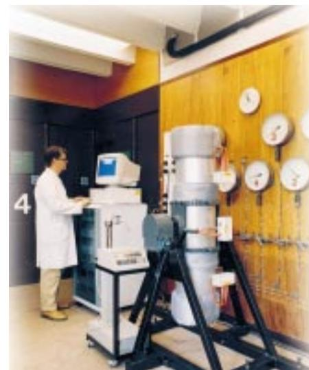
*Part of the Hydrothermal Laboratory with large flow-through autoclave in the foreground, and pressure indicators and blast-resistant cubicles in the background.*
