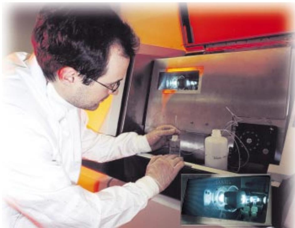
*One of the two BGS PIMMS instruments. Inset: a detailed view of the glowing argon plasma ionisation source.*
