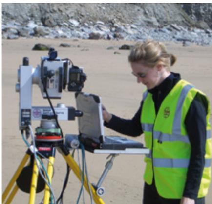
The BGS terrestrial LIDAR equipment deployed in beach surveys.
