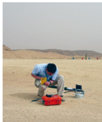
*Measuring surface gas fluxes at the CO<sub>2</sub> injection operation at In Salah in Algeria.*
