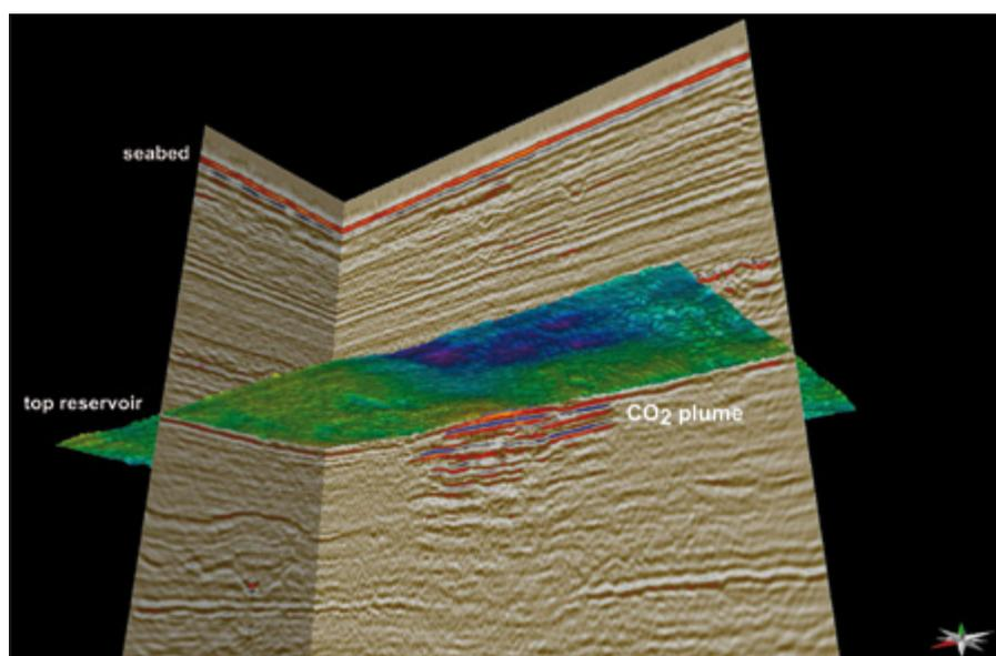
*A 3D time-lapse seismic image at Sleipner from 2006, after ten years of injection. The image shows two intersecting vertical seismic sections, the mapped top reservoir surface viewed from below and very bright reflections corresponding to the CO<sub>2</sub> trapped within the reservoir.*
