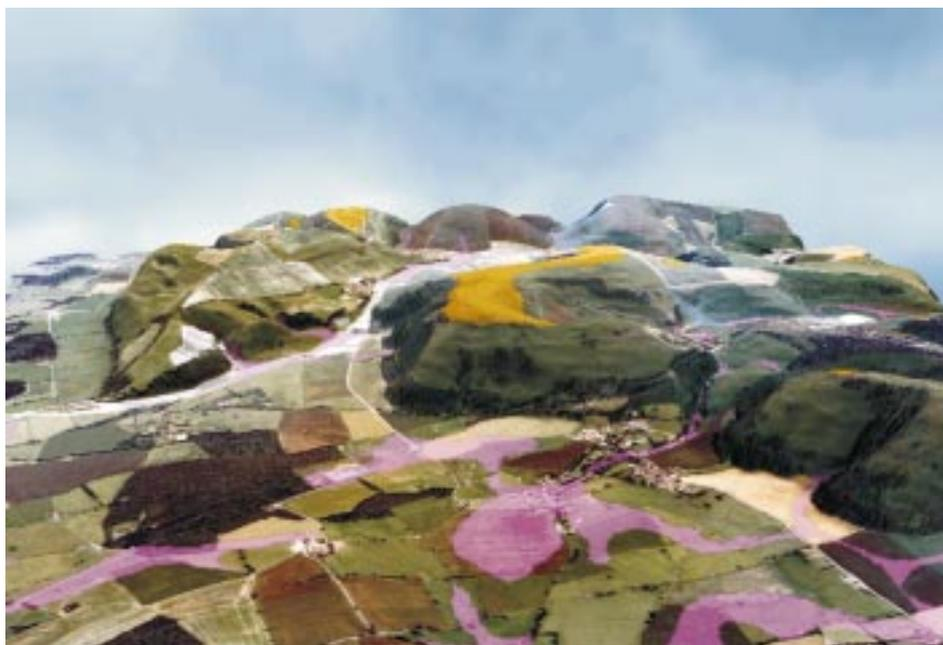
*Computer-generated perspective view of a 3D model, derived from five metre Ordnance Survey contours, draped with an orthophotograph and the drift geology as a transparent layer.*
