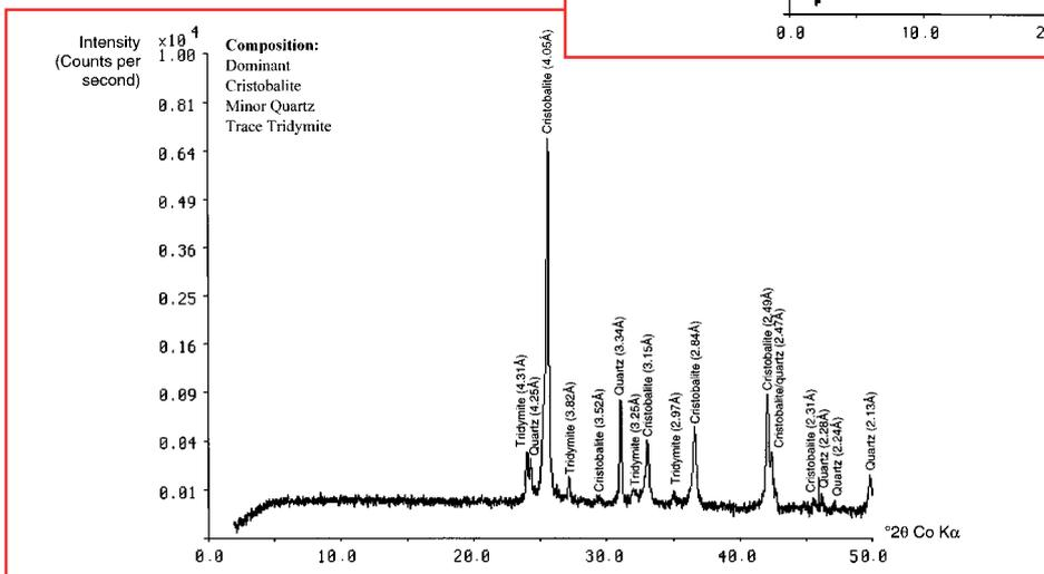
Above: X-ray diffraction profile of bulk ash sample.
