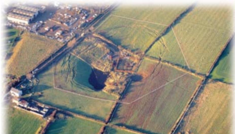
*Aerial view of the large subsidence crater formed by the collapse of Tennant Mine, Carrickfergus, County Antrim, NI. The mine was worked conventionally from the 19th Century until the 1920s and brine was extracted from it in the 1980s. It collapsed at 11.59 hours (BST) on 19th October 1990.*
