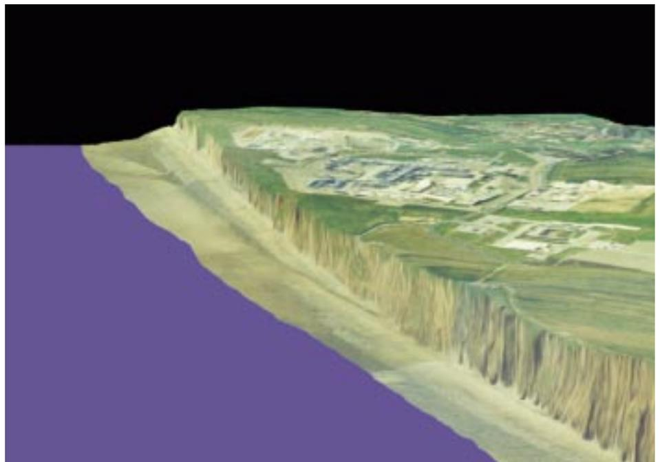
*Perspective view (looking south) of a digital terrain model (DTM) created using digital photogrammetry draped with a 2D orthophoto of the Holderness cliffs at Easington, Yorkshire.*
