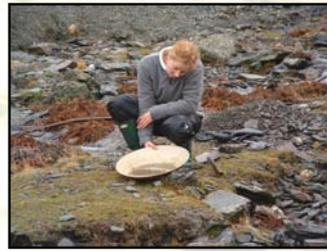
After settlement excess water is carefully drained off. The sediment is homogenised and transferred to a Kraft sample bag.
