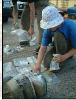
Water samples are laid out and checked off along with stream sediments and panned concentrates. Filtered waters are stored in a cool dark place prior to dispatch to BGS laboratories, while unfiltered waters are analysed daily at the field base.
