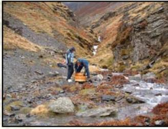
Sediment is dug from beneath the oxidised layer in the centre of the stream channel and sequentially sieved through coarse (2mm) and fine (150µm) mesh. The fine fraction is collected in a fibre glass pan and left to settle for 20 minutes.
