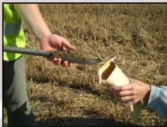
Soil samples are transferred to a Kraft sample bag prior to air drying and dispatch to the laboratories for sample preparation and analysis.
