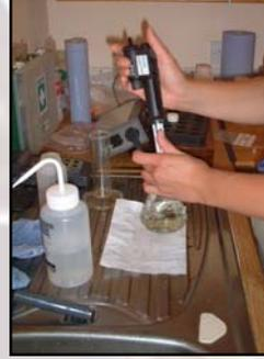
Alkalinity titrations are undertaken at the field base following pH and conductivity measurements.
