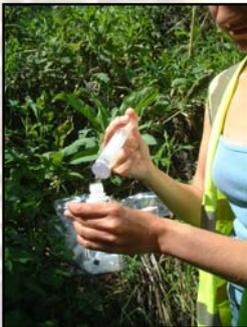
Four water samples are collected, two filtered (one acidified, one unacidified) for major and trace element analysis and two unfiltered for alkalinity, conductivity and pH determination.
