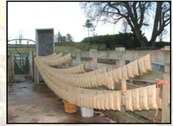
The samples are air dried until plastic in consistency, before being dispatched to Keyworth for freeze drying and sample preparation.
