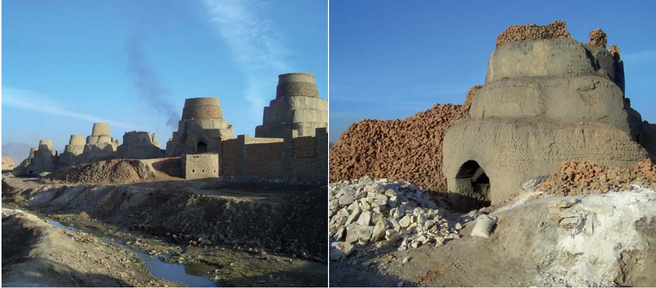
The clay deposits used for brick production, located mainly in the central and western areas of Afghanistan, are Recent, Quaternary and Jurassic in age. In Greater Kabul, there are an ever increasing number of brick kilns fuelling the demand for construction materials.
